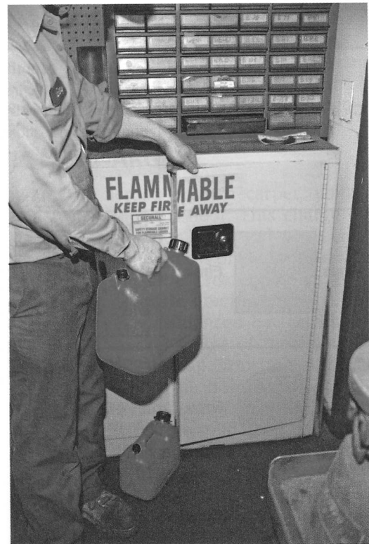
FIGURE 2-8 Store combustible materials in approved safety cabinets.
